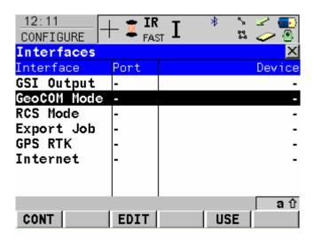
5. From the GeoCOM Mode screen verify that Use Interface is set to Yes. Change the Port setting to Port 3 (BT). Press F5 for DEVCE.
